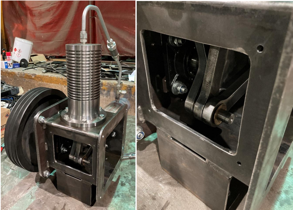
Figure 5.73: Flywheel shaft assembly fitted to engine body and crank pin inserted into hole on crank plate.
