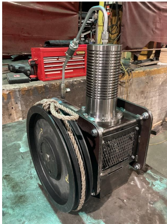
Figure 6.1: Photo of the “pull cord” wrapped around the flywheel to crank the engine.
