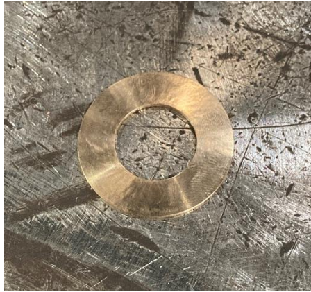
Figure 5.65: Bronze shim fabrication as per Drawing MS-SE-20.
