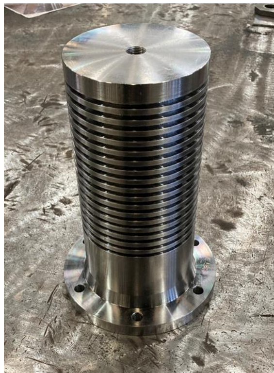
Figure 5.53: Cold cylinder fabrication as per Drawing MS-SE-02 Revision A.
