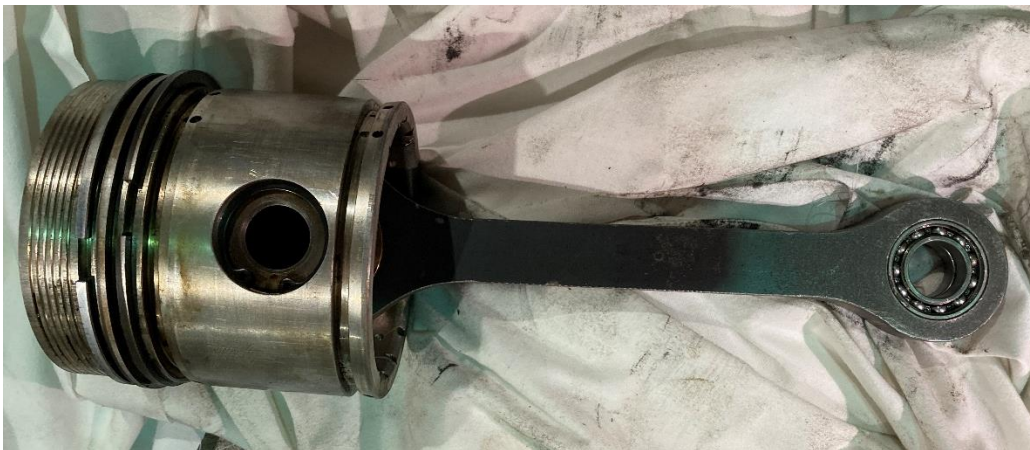
Figure 5.66: Connecting rod and piston assembly as per Drawing MS-SE-16.
