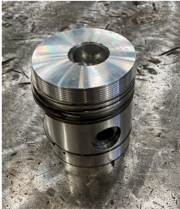
Figure 5.9: Lister 18018 000T1 piston for Stirling engine prototype.
