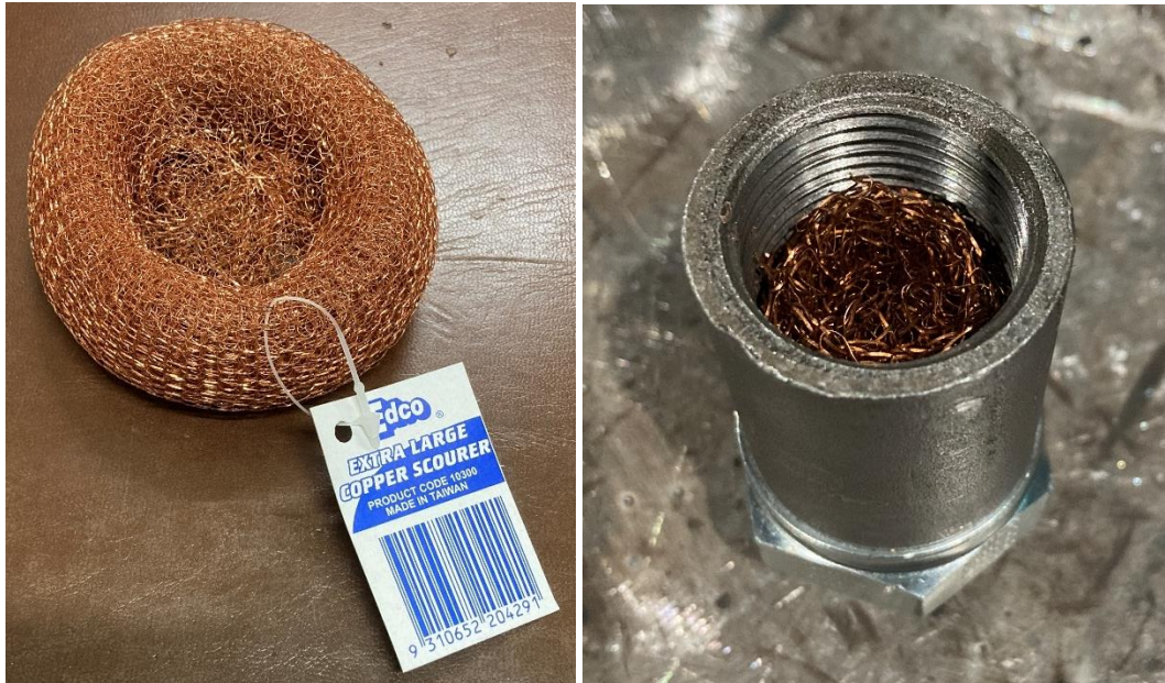
Figure 5.12: Copper scourer utilised for the regenerator matrix.
