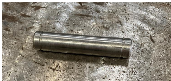
Figure 5.56: Crank pin fabrication as per Drawing MS-SE-05.
