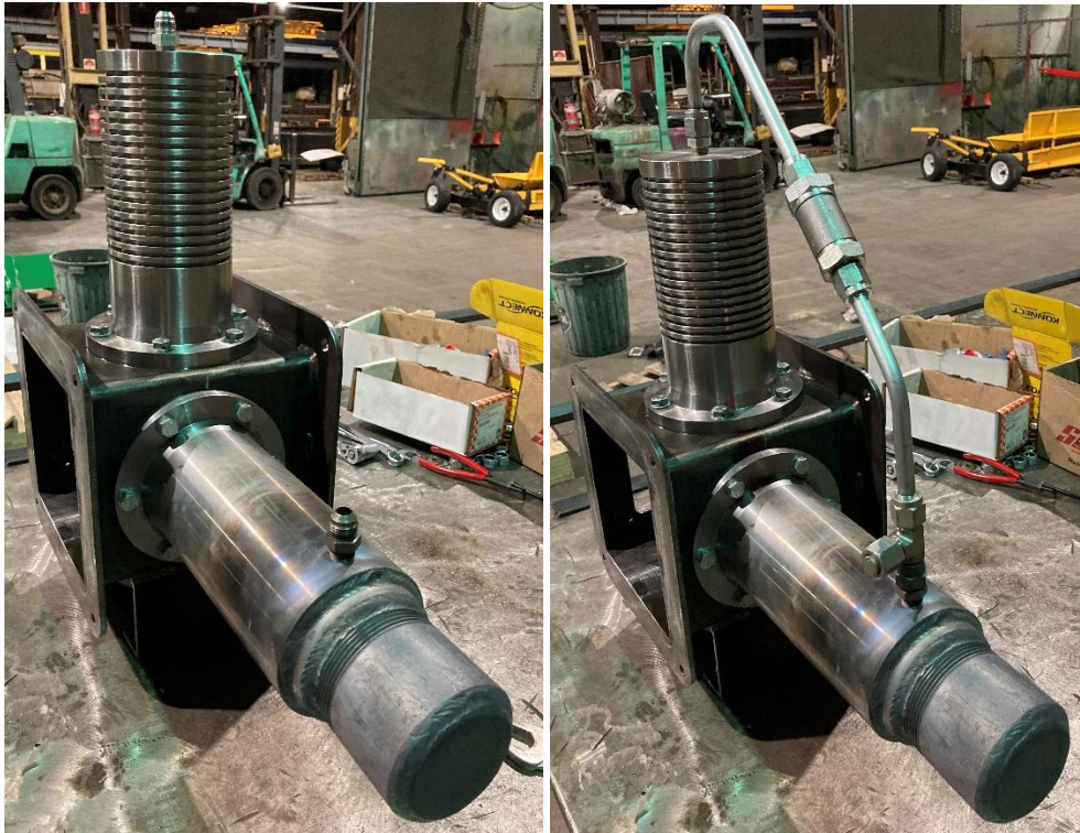
Figure 5.71: Assembly of cylinder assemblies onto engine body and air tube fitted to cylinders.
