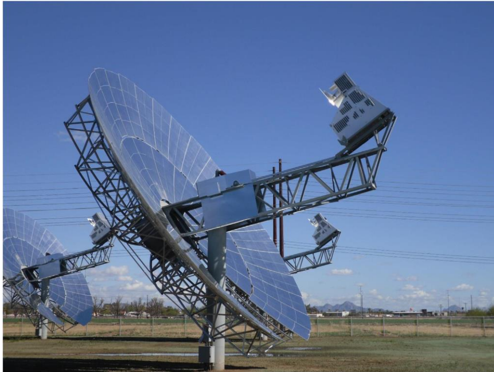
Figure 2.30: Concentrated solar dish with Stirling engine mounted at focal point (Boretti 2021, pp. 16241-16247).
