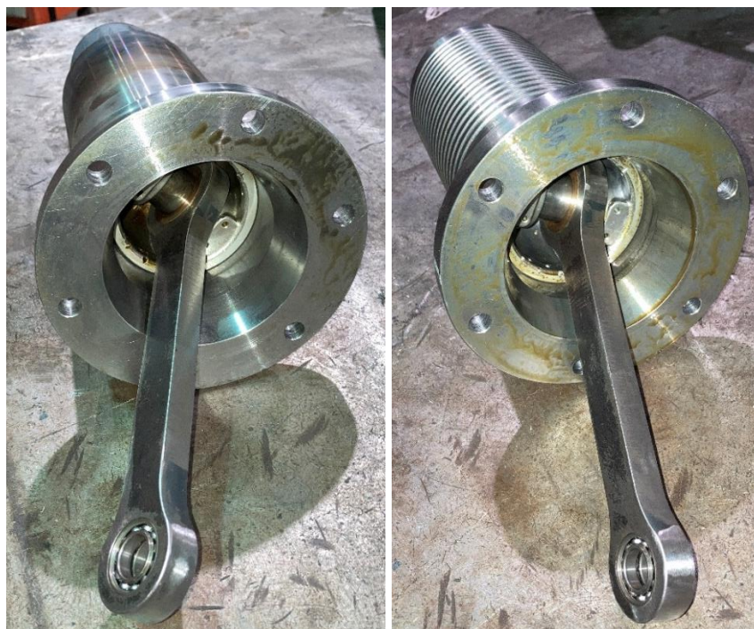
Figure 5.70: Assembly of piston and connecting rod assemblies in hot and cold cylinders.
