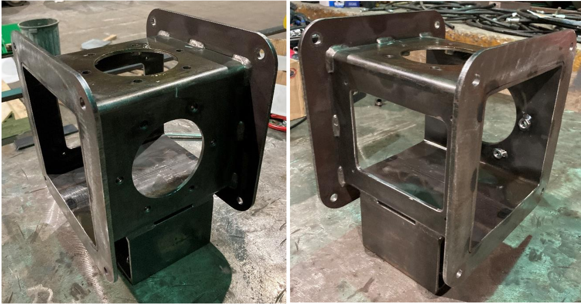
Figure 5.54: Engine body fabrication as per Drawing MS-SE-03 Revision B.
