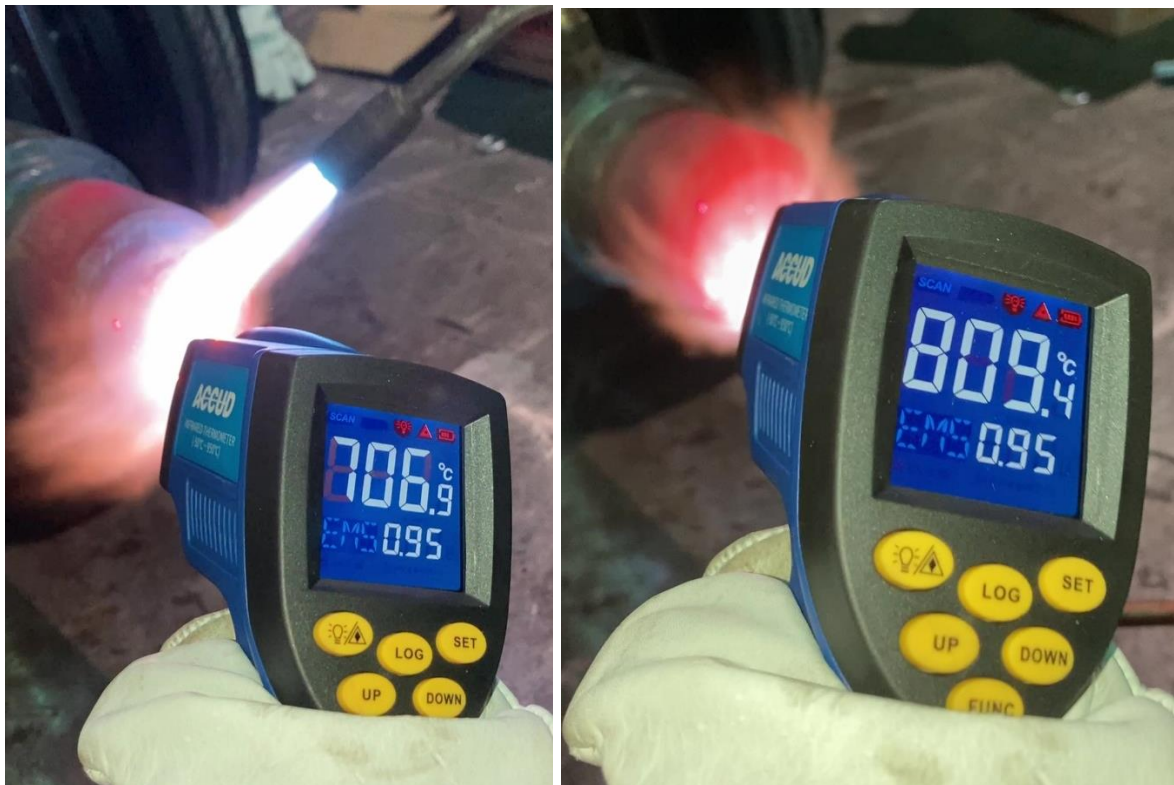
Figure 6.6: Heater head heated to 700° C and 800° C during testing.
