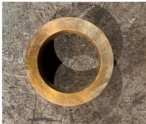
Figure 5.58: Bronze bush fabrication as per Drawing MS-SE-08.
