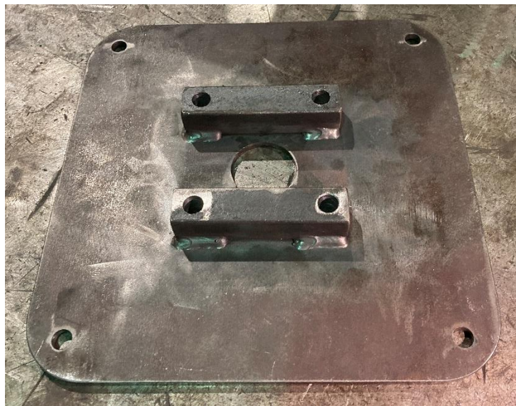
Figure 5.55: Bearing plate fabrication as per Drawing MS-SE-04.
