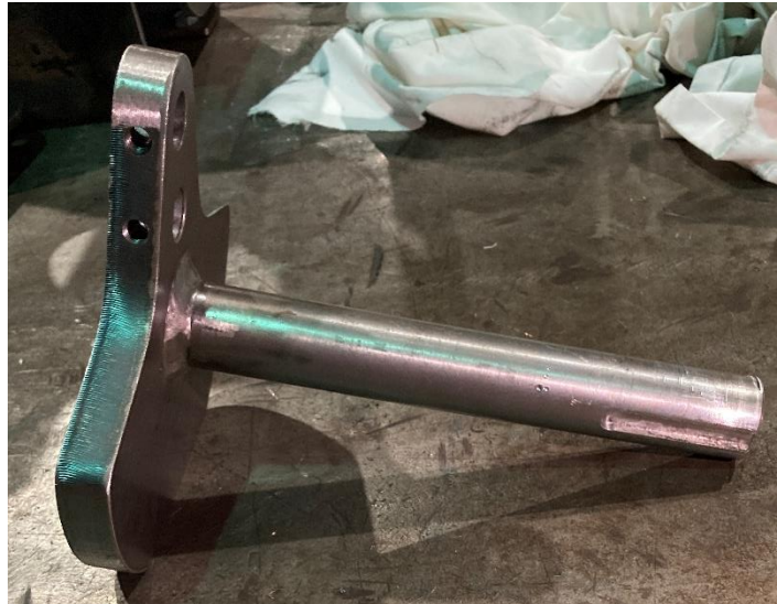
Figure 5.62: Idler shaft and crank plate fabrication as per Drawing MS-SE-13 Revision B.
