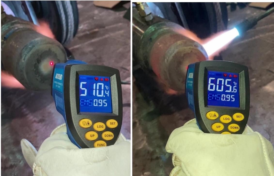
Figure 6.5: Heater head heated to 500° C and 600° C during testing.
