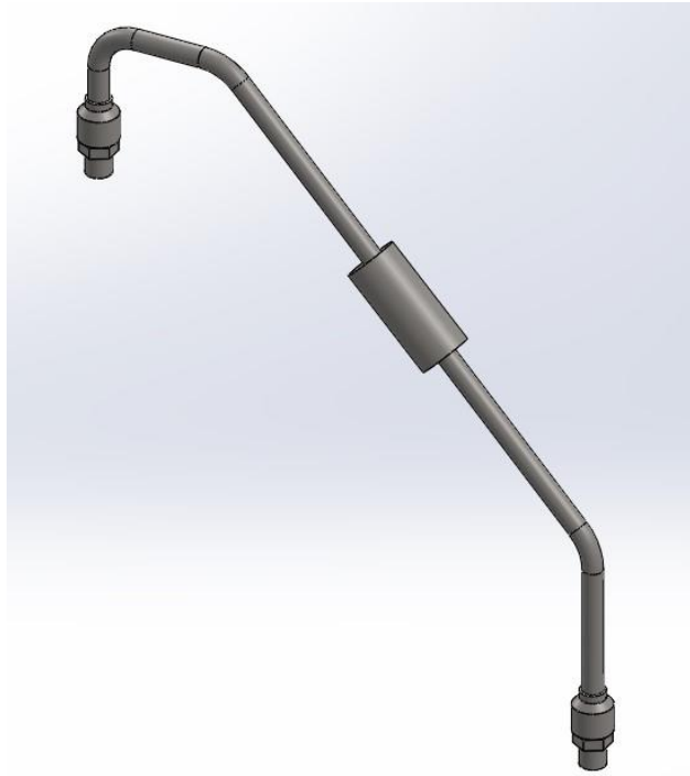
Figure 5.11: Connecting air tube solid model.
