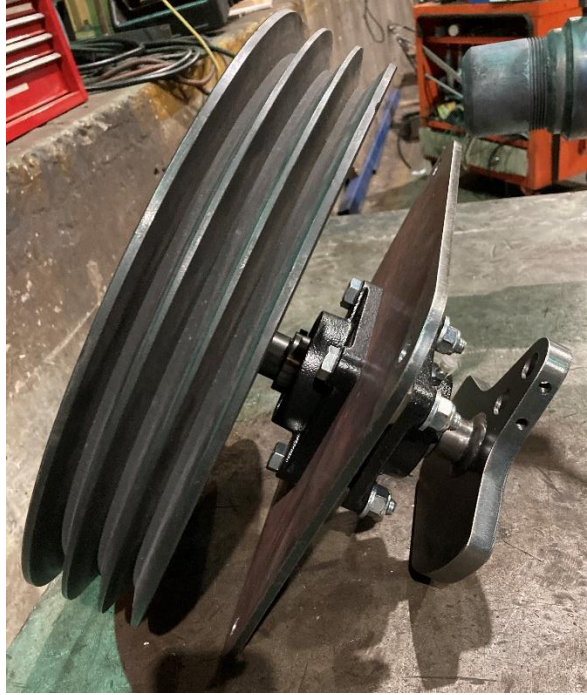
Figure 5.67: Flywheel shaft assembly as per Drawing MS-SE-17.
