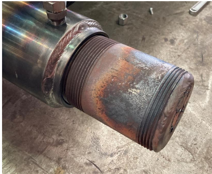
Figure 5.69: Heater head fitted to hot cylinder.
