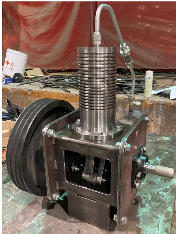
Figure 5.74: Output shaft assembly fitted to engine body and crank pin inserted into hole on crank plate.
