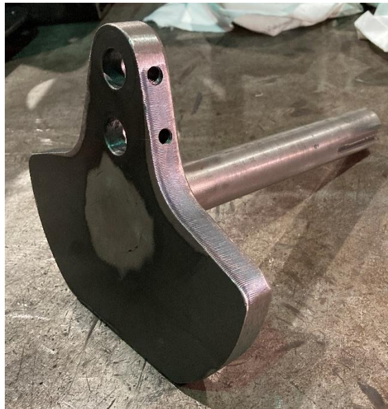
Figure 5.61: Output shaft and crank plate fabrication as per Drawing MS-SE-12 Revision B.
