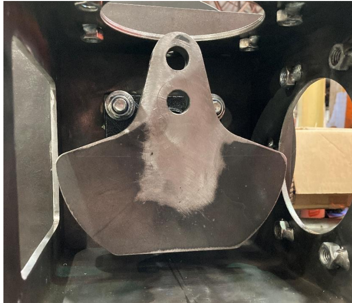
Figure 6.3: Second hole drilled in crank plate for crank pin at 42 mm from the centre of the output shaft.
