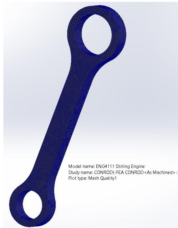
Figure 5.30: Meshed connecting rod for analysis.
